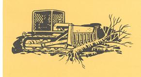
Rake is installed and held by two pins and brackets which are installed on the top end of moleboard of blade.
